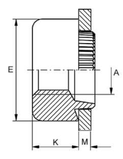
Female thread A = M16Height K = 10.0Outer diameter E = 25.0Plate thickness = 4.7 to 4.9
